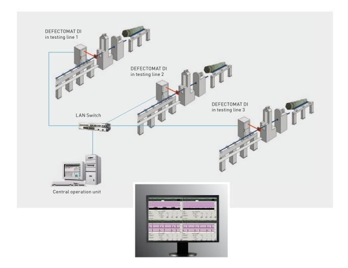
The DEFECTOMAT DI integrates all necessary functions and interfaces for eddy-current testing, and permits the connection of maximum two test coils or probes. The compact dimensions of the DEFECTOMAT DI allow close integration to the testing line.
