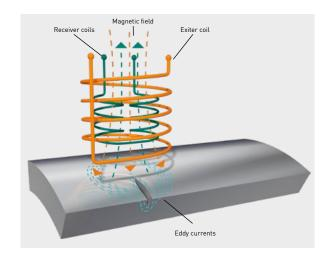
Figure 6: The principle behind eddy current testing
