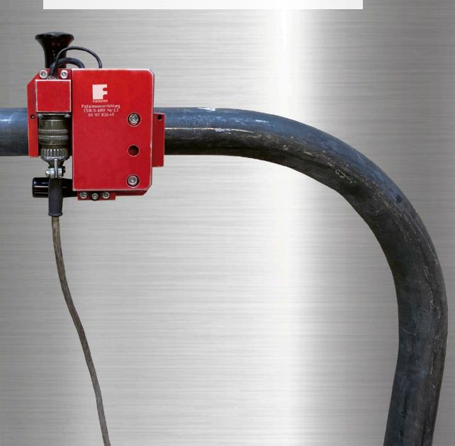
Wrought outlet pigtails are critical components that need rigorous inspection due to their location and intended function. For the identification and determination of creep, we have developed a unique device for measuring pigtails diametrically from the tube outlet to the manifold.
