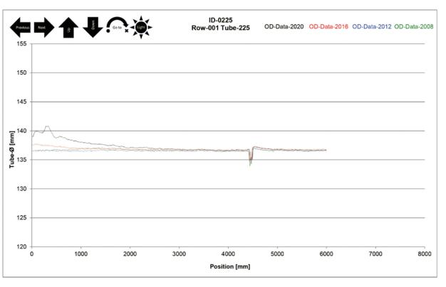
$Figure\ 2: Four inspections\ of\ a\ reformer tube's\ outside\ diameter\ are\ superimposed\ to\ show\ changes\ over\ time\ (baseline\ taken\ in\ 2008\ and\ inspections\ in\ 2012,\ 2016\ and\ 2020)$
