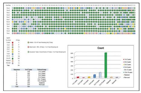
Figure 5: Typical output for the Remaining Life Assessment
