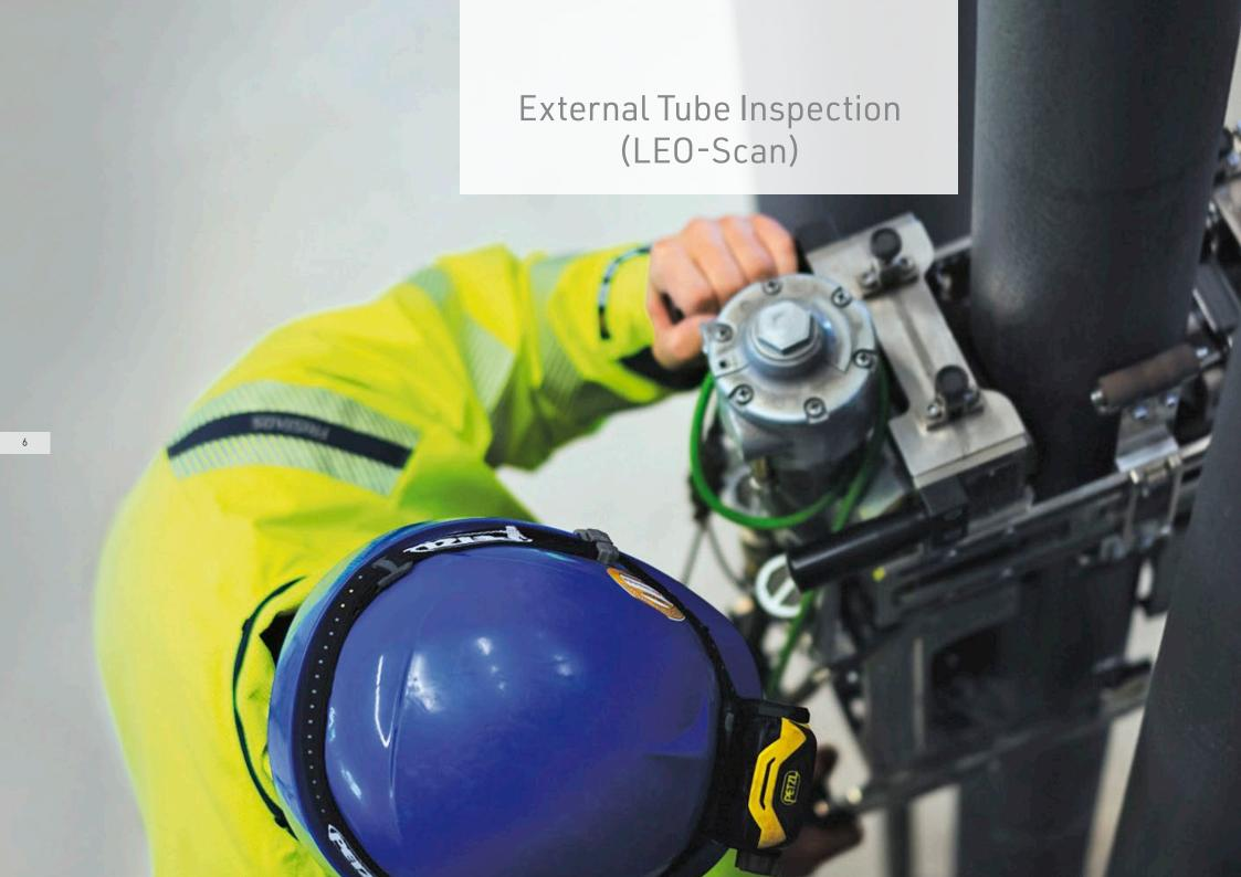
For the purpose of inspecting centrifugally cast reformer catalyst tubes used in steam methane reformers, FOERSTER has developed and built the proprietary "LEO-Scan" system, an inspection carried out from the outside of the tubes, using the Eddy current and Laser technique.
